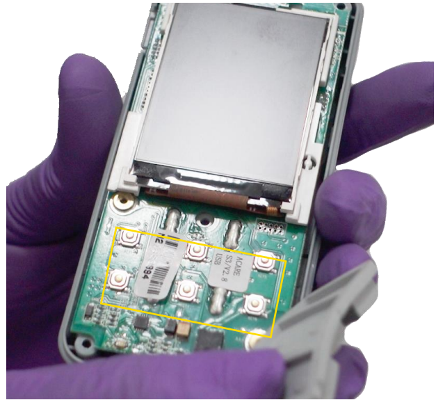
7.11 Check the keys for water damage.
