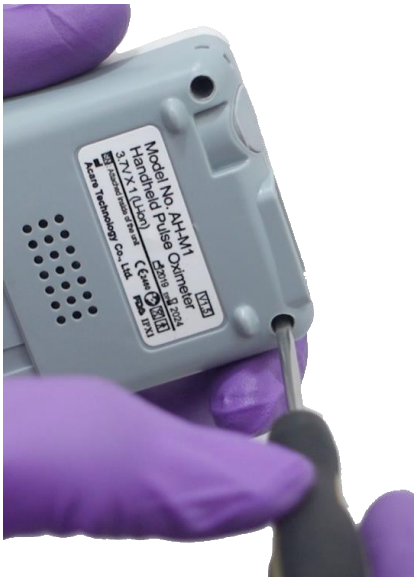
7.5 Unscrew the back of the pulse oximeter.
