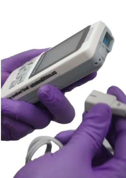
7.2 Remove probe by base connector.
