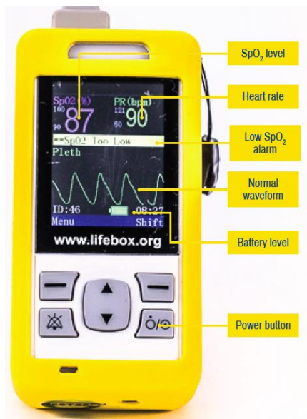
2.5 Main external components of a pulse oximeter.
