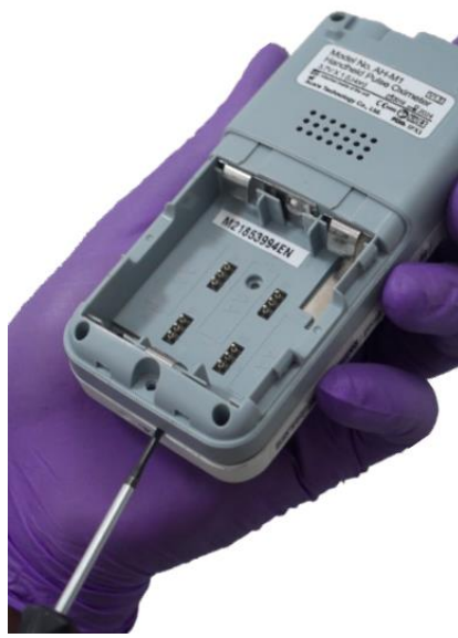
7.6 Gently pry off the back housing.
