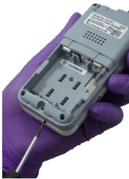
7.6 Gently pry off the back housing.
