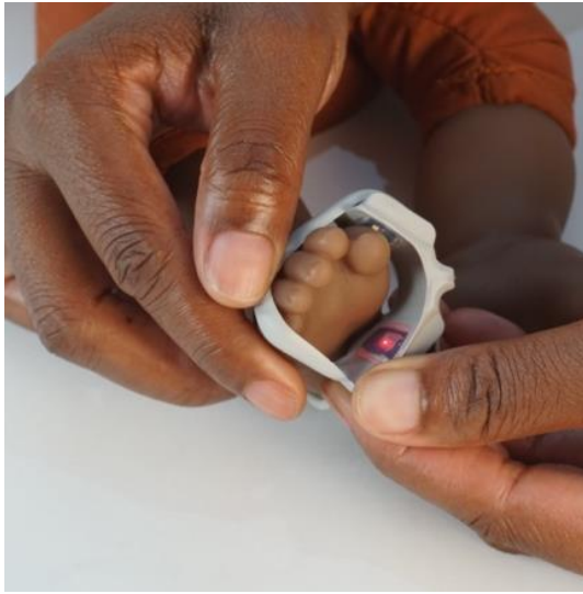
3.5 Wrap rubber connecting strip around foot.
