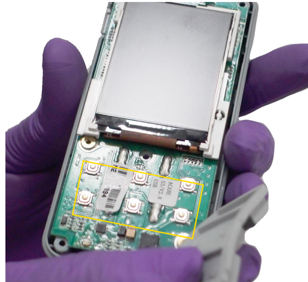
7.11 Check the keys for water damage.
