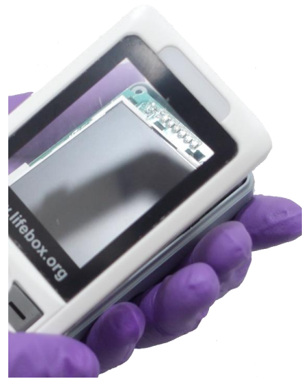
7.7 Open pulse oximeter to view components.
