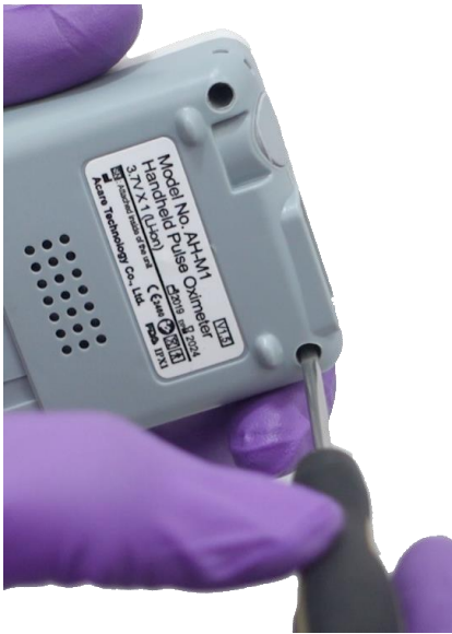
7.5 Unscrew the back of the pulse oximeter.
