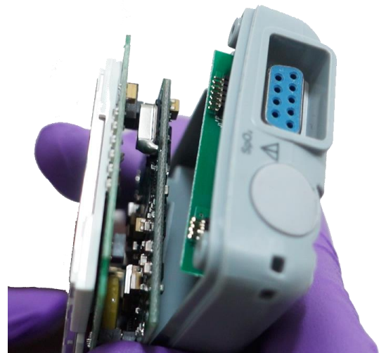
7.9 Gently pull up circuit boards to replace.
