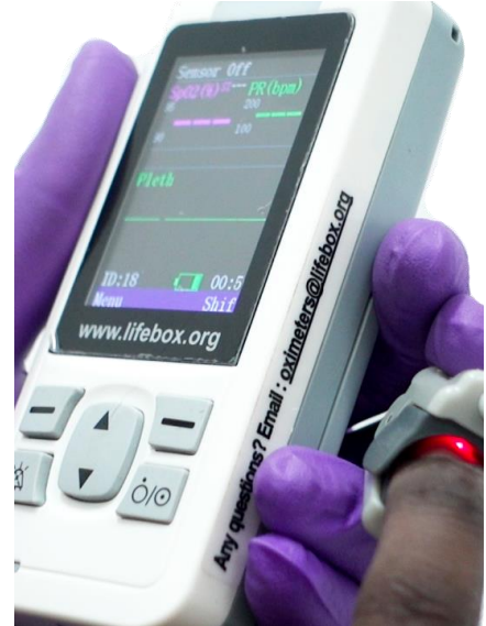
7.4 Not all probes will work with all pulse oximeters.
