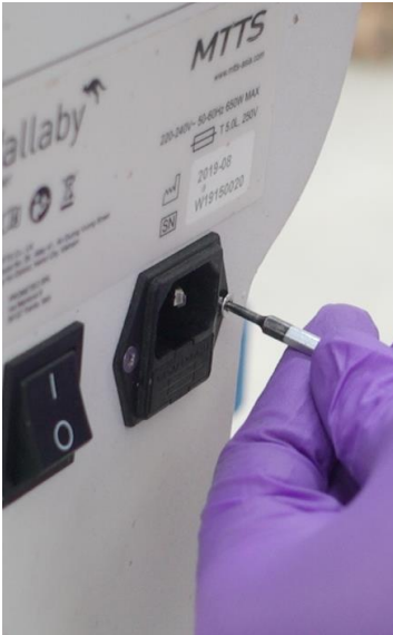
7.13 Unscrew power supply module from housing.
