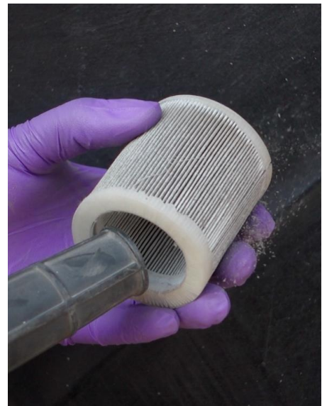
7.14 Dust should blow off the filter paper.
