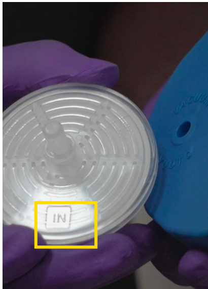
7.15 Check direction before inserting filter.
