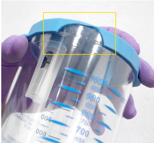
7.7 Assess the collection reservoir for cracks.
