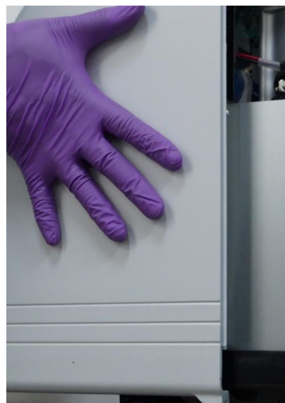
7.3 Unscrew and slide the front housing off of the device.
