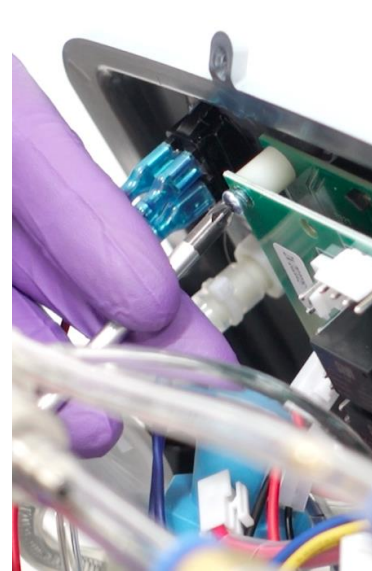
7.6 Unscrew the circuit boards from the concentrator housing. Replace as needed.
