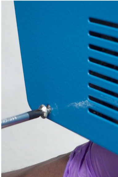
7.9 Unscrew housing to access the pump.
