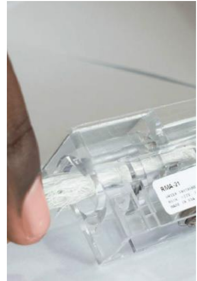
7.14 Insert the cleaning rod in the flowmeter barrel and clean.
