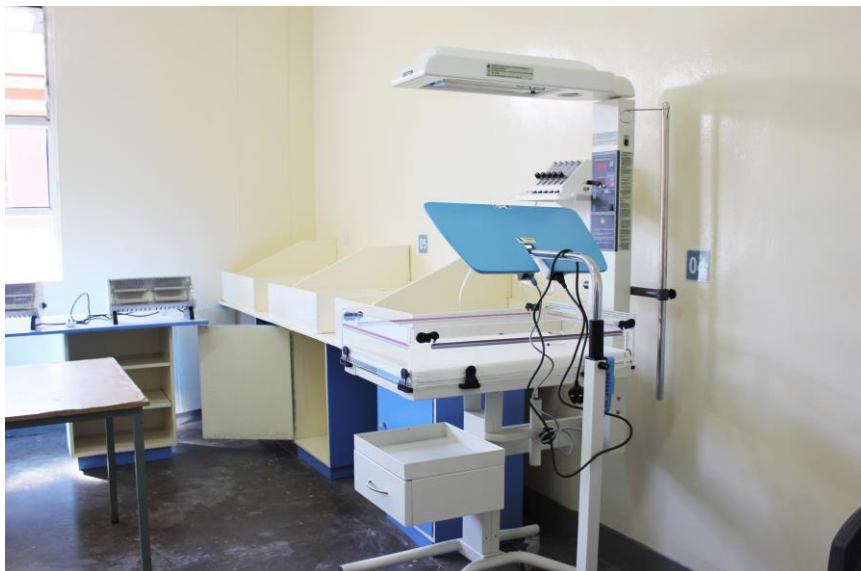
6.3 Appropriate placement with the power cable port facing the wall and display LCD facing away from the wall.
