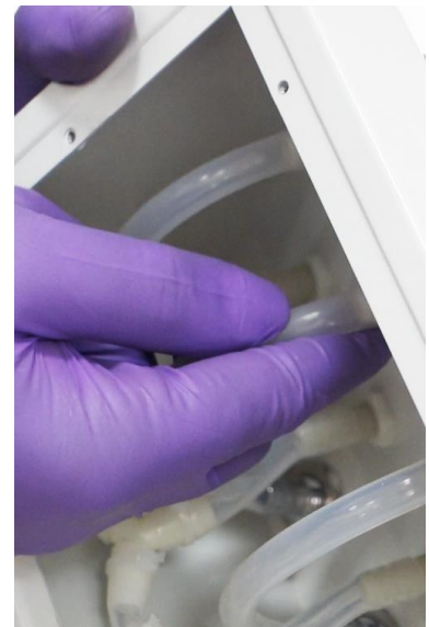
7.4 Remove flow meter and clean or replace.
