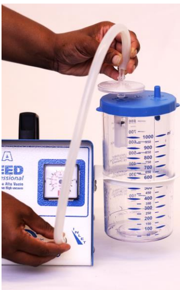
3.3 Connect short tubing to filter & inlet port.
