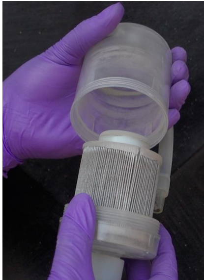
7.11 Unscrew and separate the two parts of the plastic housing for the filter paper cylinder.
