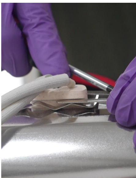
7.19 If replacing, remove clip securing the element.
