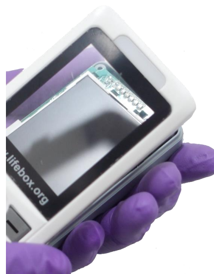
7.7 Open pulse oximeter to view components.
