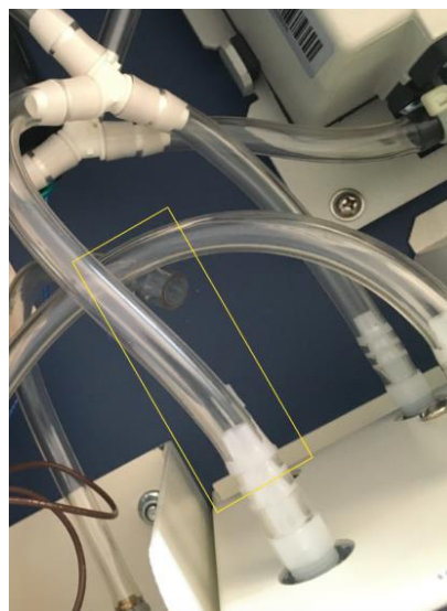
7.2 Displaced internal tubing.
