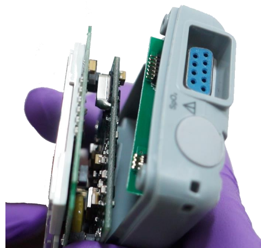
7.9 Gently pull up circuit boards to replace.
