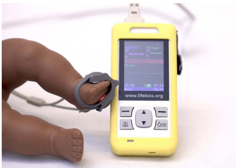
2.2 SpO 2 levels should be monitored regularly and remain between 90 – 95%.
