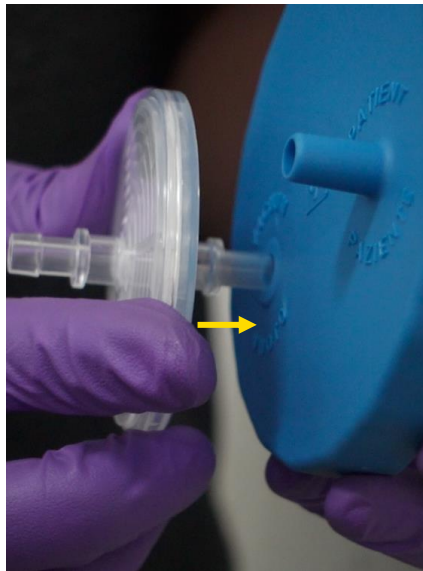
7.16 Gently insert filter into the "Vacuum" port.
