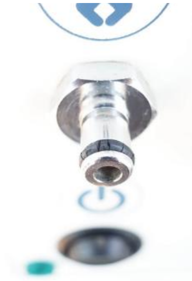
7.4 Deteriorating patient port seal.
