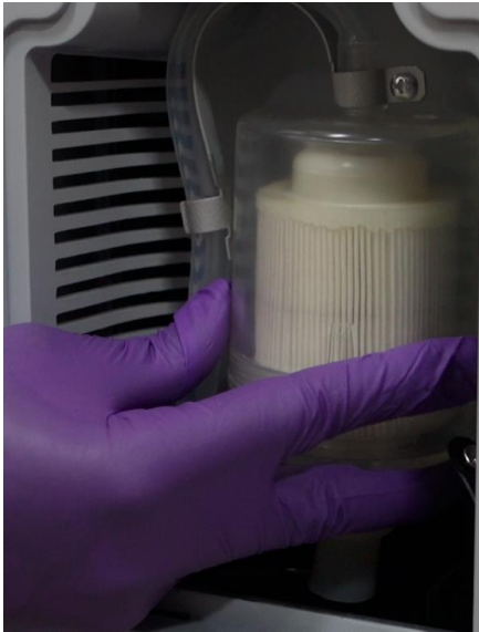
7.10 Remove the fine particle intake filter from the concentrator.
