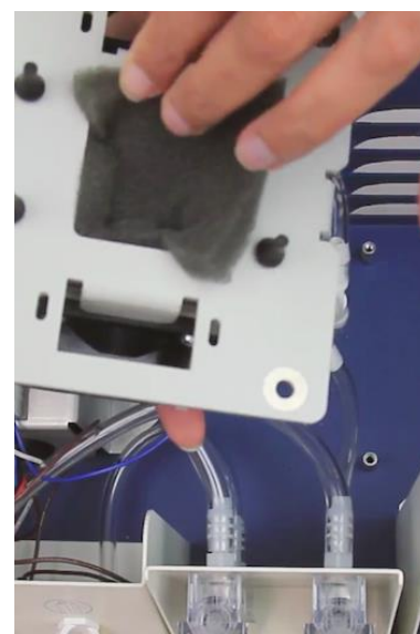
7.7 Push in the replacement pump filter until it fits flush to the housing.
