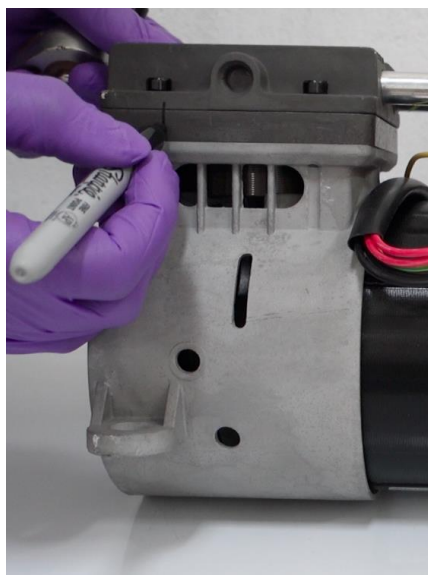
7.20 Mark sides of the compressor.
