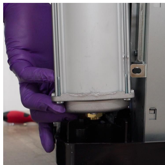
7.18 Replace the sieve beds in pairs, following grooves along sieve bed housing to snap into place.
