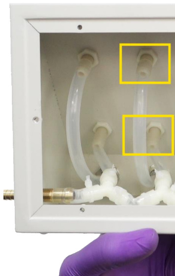
7.3 Disconnect flow meter at inlet and outlet barbed connectors.
