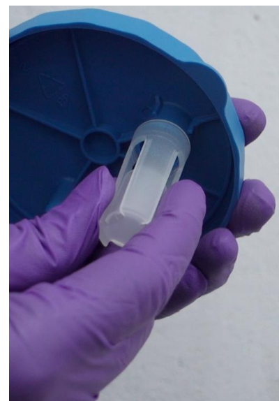
7.6 Float valve installation: push in until firmly secured.
