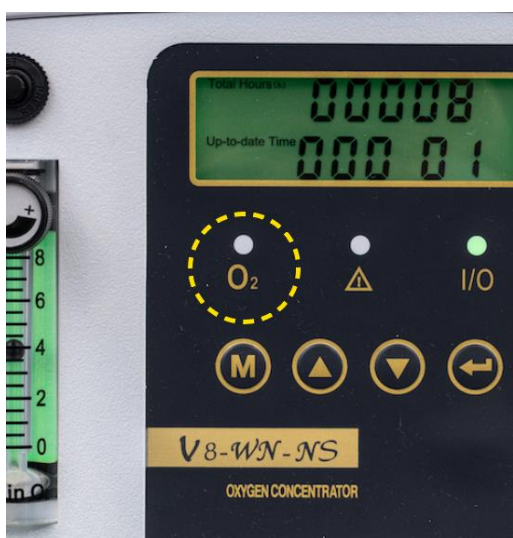
3.2 The “Low Oxygen” alarm indicates that produced concentrations are lower than 85%.
