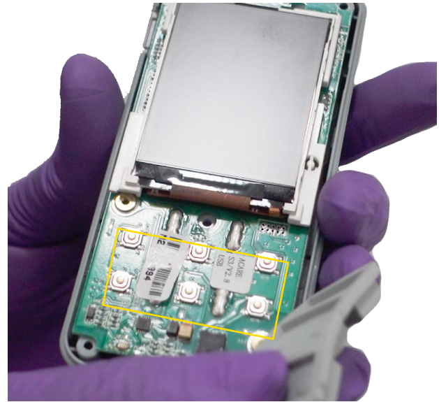
7.11 Check the keys for water damage.
