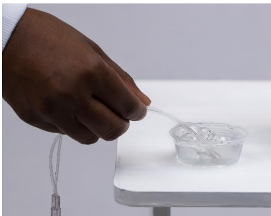
3.1 Submerging the nasal prongs in water should produce bubbles.
