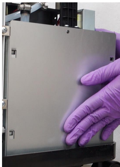
7.19 Slide panel up to access compressor.
