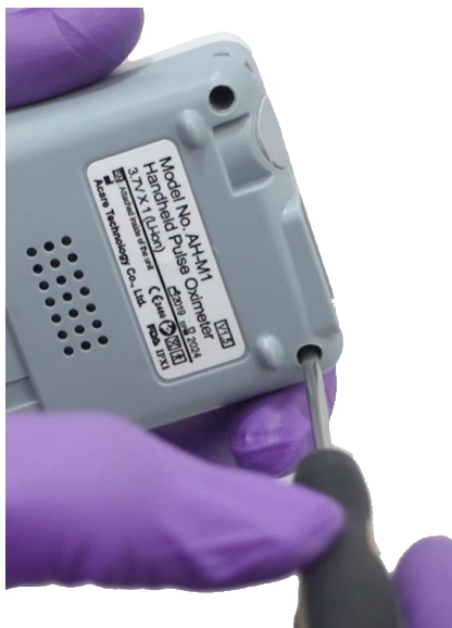
7.5 Unscrew the back of the pulse oximeter.
