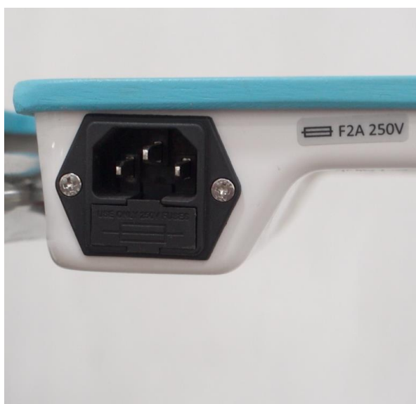
7.1 Assess the housing for fuses.
