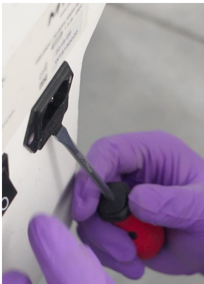
7.1 Use a screwdriver to open the fuse drawer.
