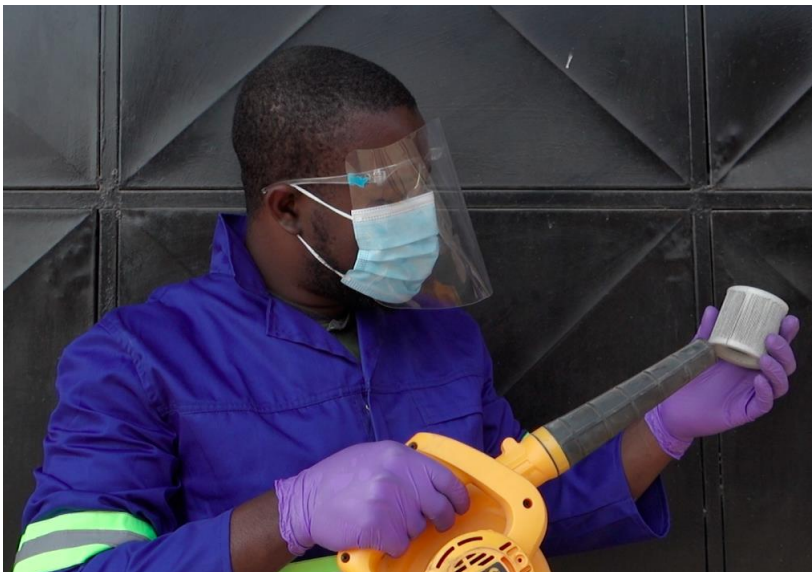
7.13 Wearing PPE and using compressed air, clean all components of the fine particle intake filter separately.
