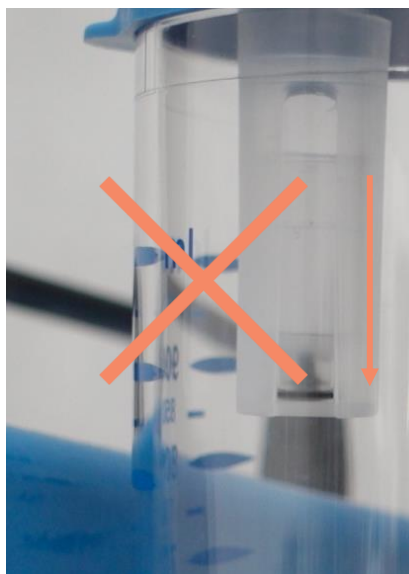
7.5 Incorrect float valve orientation.
