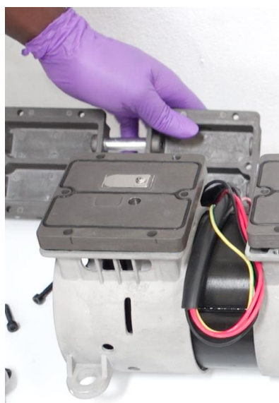
7.22 Lift off compressor head & assess head gaskets for damage.
