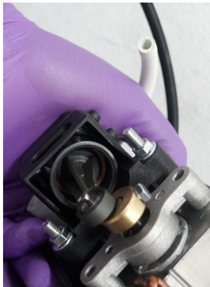
7.13 Inspect pump assembly for damage to components.
