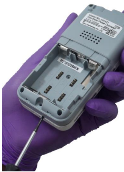
7.6 Gently pry off the back housing.
