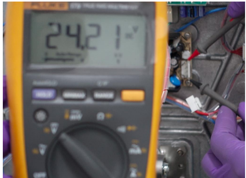
7.7 Test known voltages along the power supply unit and throughout the wiring circuits.
