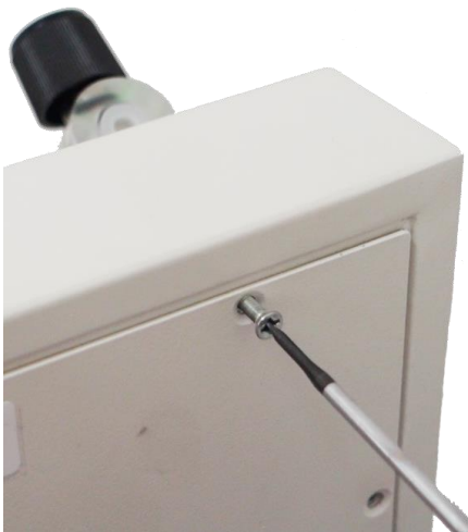
7.2 Open housing to access internal tubing.
