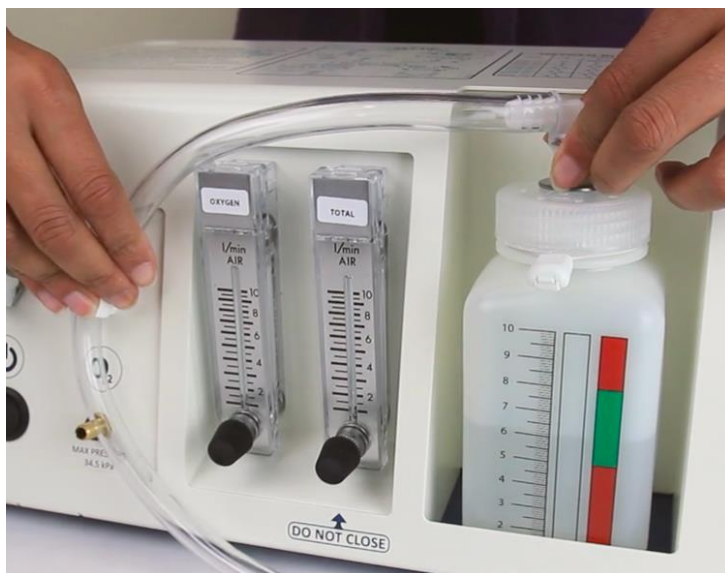
3.6. Connect & brace long expiratory tubing in bottle bracket
