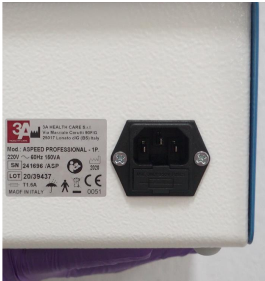
7.1 Assess the housing for fuses.
