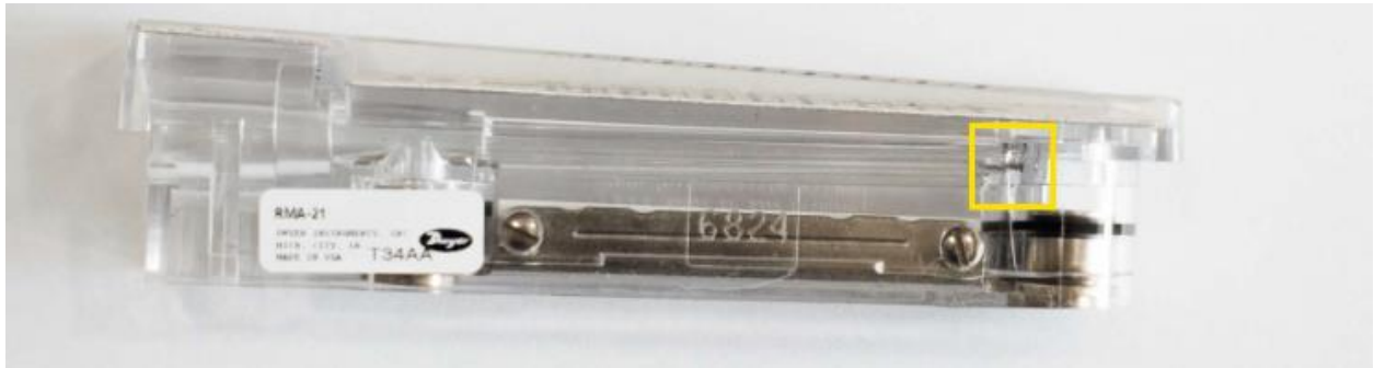
7.8 Debris development in the base of the flowmeter channel
