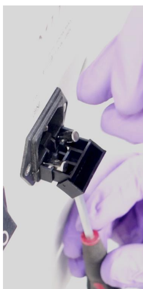
7.4 If replacement is needed, remove the faulty fuse.
