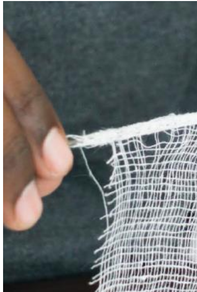
7.13 Prepare a cleaning rod by wrapping a wire with gauze.
