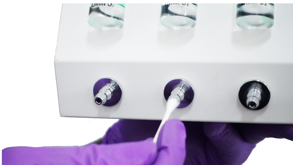
7.1 Clean debris from outlet ports with an ear swab soaked in 70% alcohol.
