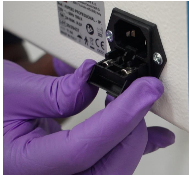
7.2 Open the fuse drawer and inspect the fuses. Test with a multimeter.
