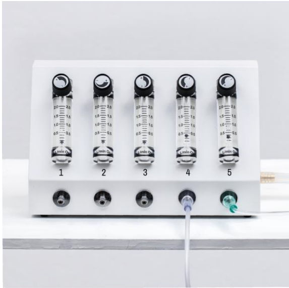
3.1 The oxygen splitter is securely placed with easy access to flow meters.
