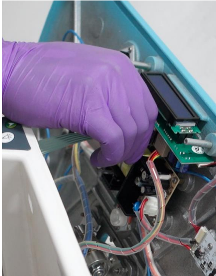
7.8 Check that components are securely connected to the PCBs.
