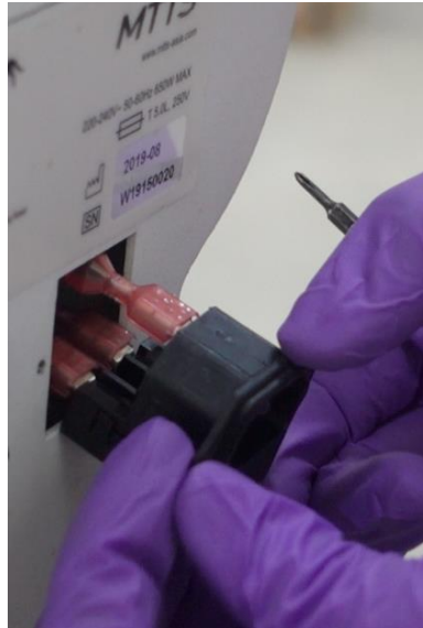
7.14 Pull the module from the housing.
