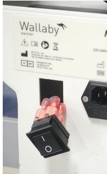
7.8 Pull out the power switch to access switch terminals.
