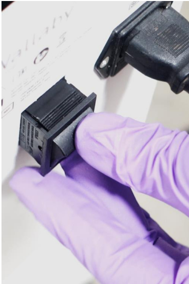
7.7 Remove the power switch from the housing.
