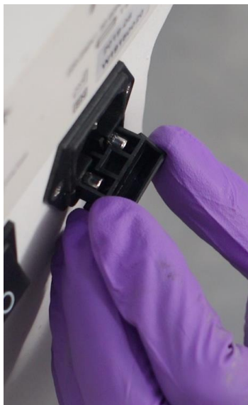
7.2 Pull out the fuse drawer to view the fuses.
