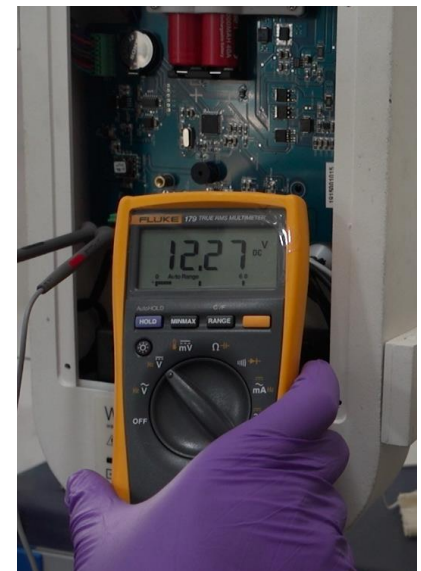
7.12 Confirm voltage at the PCB power supply with specifications.
