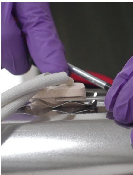
7.19 If replacing, remove clip securing the element.
