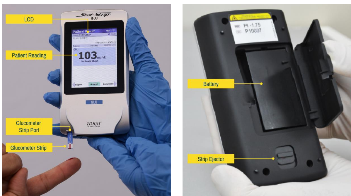
2.3 Glucometer main components.
