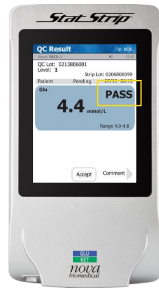
6.5 The control solution should test as a Pass .
