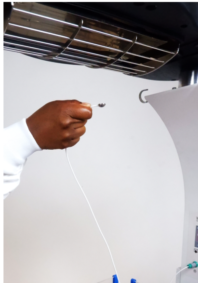
3.5 Pass the temperature probe underneath the heating elements.
